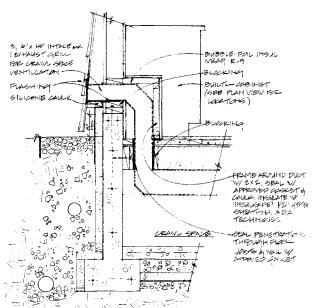
Fig. 3. Crawl space ventilation detail.
